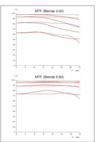
The MTF is indicated both at full aperture and at f/5.6 at long taking distances (infinity). Shown is the contrast in percentage for 5, 10, 20 and 40 lp/mm accross the height of the 35 mm film format, for tangential (dotted line) and sagittal (solid line) structures, in white light. The 5 and 10 lp/mm will give an indication regarding the contrast ratio for large object structures. The 20 and 40 lp/mm records the resolution of finer and finest object structures.
